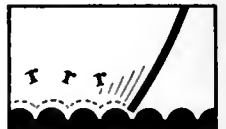
This is the action of the usual wirewound control after it has been in use for some time . . . like dragging a stick over a cobblestone pavement.
