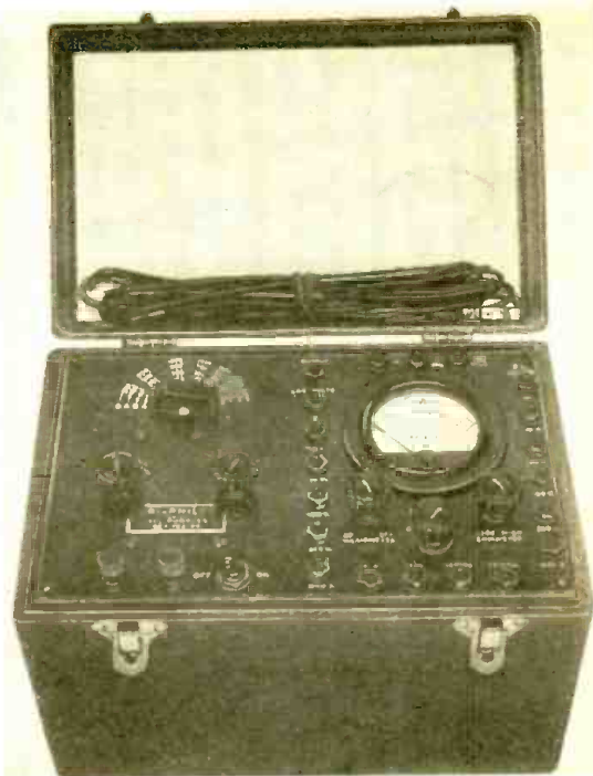
Panel view of the N. R. I.—Philco set tester described here.
