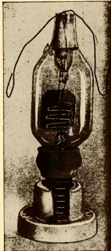
Courtesy R. McV. Weston, F.R.P.S. A 1907 audion, once owned by J. A. Fleming.
