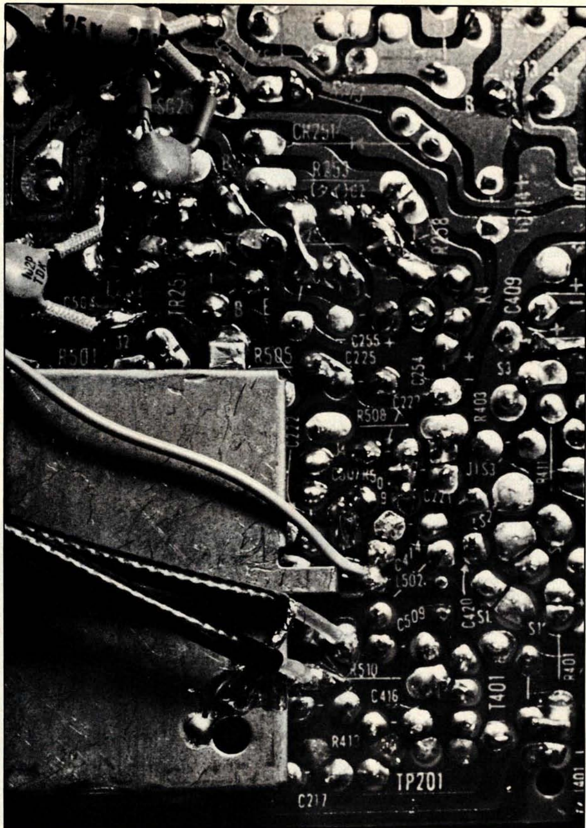
Photo 5: This view shows where modifications must be made to the underside of the Hitachi SX chassis printed circuit board. A foil trace carrying the video signal is cut and routed through shielded wire to the external switch, and a small disk capacitor (at top with spaghetti tubing on legs) is attached across a spark gap to improve the set's response to abrupt black and white changes.
