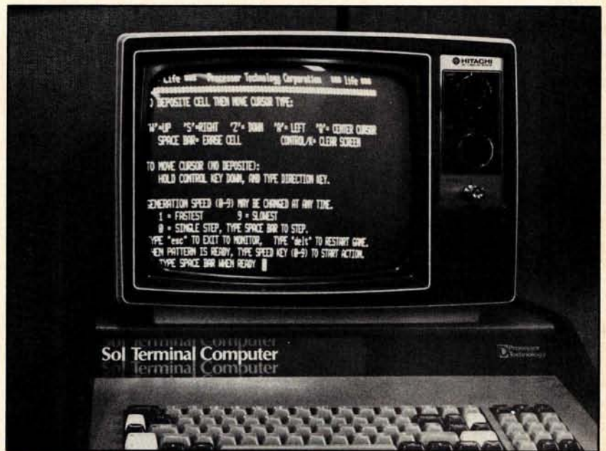
Photo 7: To illustrate the wider field possible with the Pickles and Trout direct video conversion, the 64 character display of a SOL-20 was used with the converted television perched on top of the SOL. We made no attempt to adjust the controls of the television set to remove the overscan condition evident in this photo of the Processor Technology LIFE demonstration program's output.
