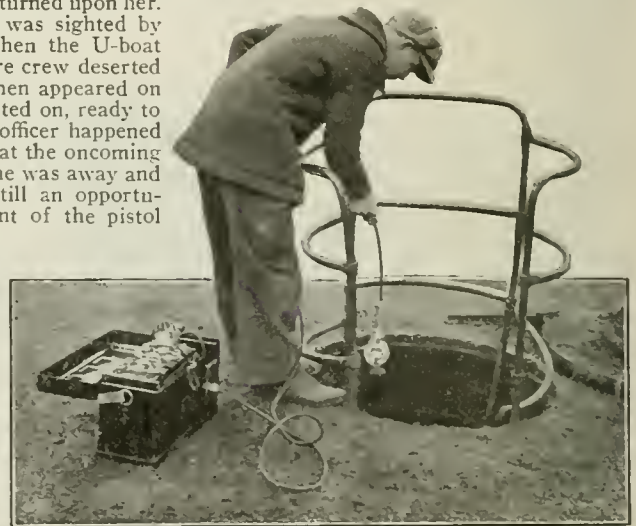
For Lighting Manholes, Cable and Pipe Tunnels, and a Hundred Other Places, This New Storage Battery Lighting Outfit Will Prove Ideal.
