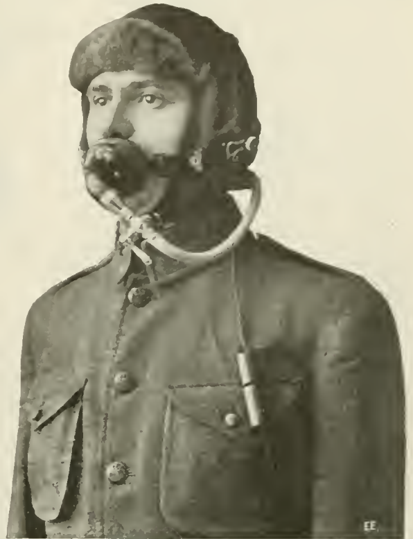
U. S. Aviators Are Being Supplied With the New Dictograph Here Shown, for Carrying on Conversation With a Second Officer, While in Flight. The Engine Noise and Wind Make It Difficult to Talk Otherwise.
