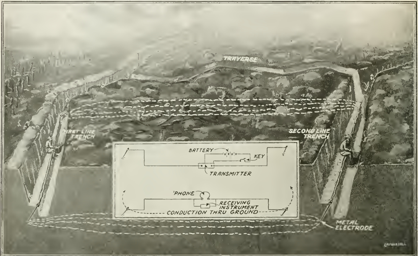
A New "Wireless" Communication Scheme Is Now Being Used In the French Front Line Trenches. This Is Nothing More Nor Less Than "Ground Telegraphy" in a New Dress. By Using Specially Tuned Transmitters and Screens, Interference By the Enemy Is Practically Eliminated.
