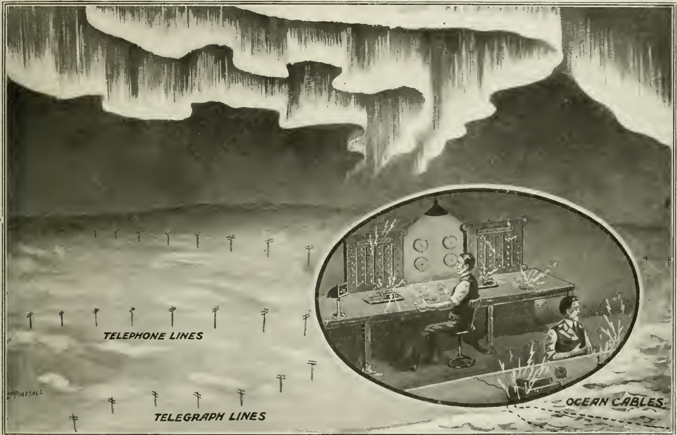
The "Aurora Borealis" Visits Us Every Now and Then, the Last One Having Occurred on August 9, 1917. At These Times There are Severe Electrical Disturbances Set Up on Telephone and Telegraph as Well as Cable Lines. Transient Electric Currents Often Surge Thru the Circuits, Which Register a Potential of Several Hundred Volts.
