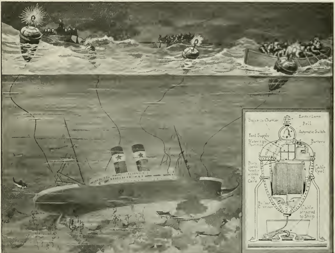
One of Uncle Sam's Naval Men Has Suggested a New Salvaging Scheme for Saving Sunken Ships. He Proposes to Equip Every Boat with a Series of Electrical Buoys, which Rise when the Ship Sinks. These Buoys Carry Cables From the Ship, and May Carry Electric Lights as Well as Food for the Survivors.
