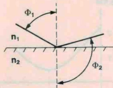
with different refractive indices. Between air and water is one such boundary. Between air and glass is another. It's also possible to make different types of glass, with different refractive indices.
