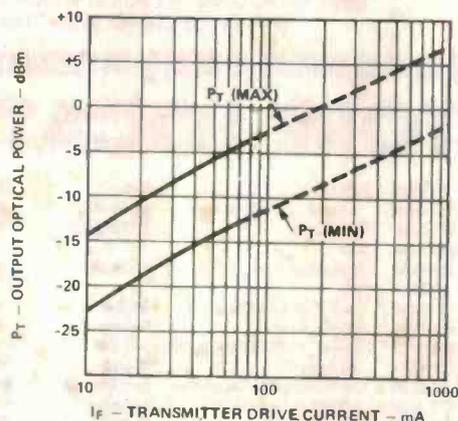
value of resistor R needs to be calculated. This is a simple procedure, as follows. First determine the maximum and minimum output levels for the transmitter. The equation is given on page 10 of the HP data sheets but can be simplified to:
