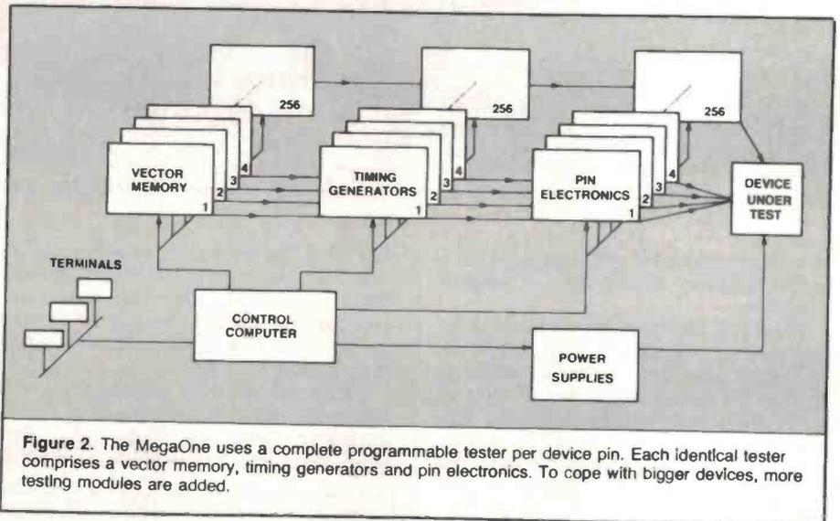
Figure 2. The MegaOne uses a complete programmable tester per device pin. Each identical tester comprises a vector memory, timing generators and pin electronics. To cope with bigger devices, more testing modules are added.
