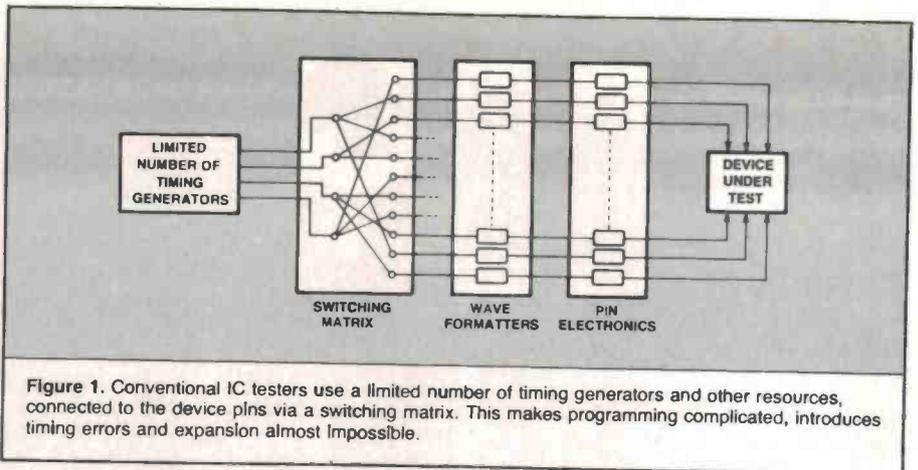
Figure 1. Conventional IC testers use a limited number of timing generators and other resources, connected to the device pins via a switching matrix. This makes programming complicated, introduces timing errors and expansion almost impossible.
