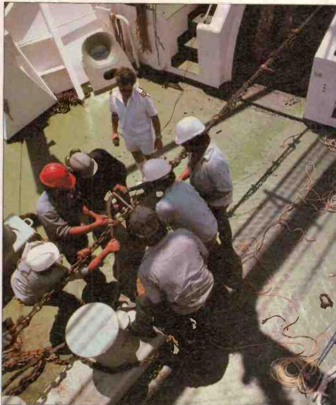
Above. Securing an end of cable even more firmly once on board. The cable can then be pulled inside the ship for testing or repairs. Below. The cable is hauled across the deck then over large drums to be fed into a series of hydraulic wheels and out to the working area.
