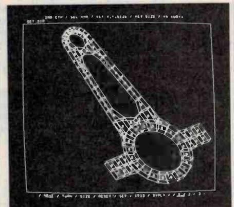
A typical CAD 'wire' drawing. Courtesy AUSTCAD.
