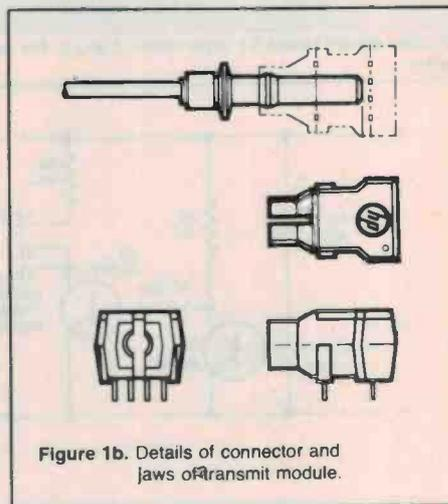
Figure 1b. Details of connector and jaws of transmit module.
