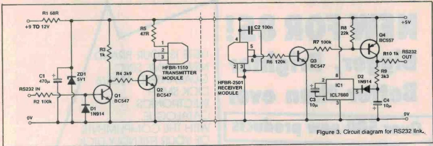
Figure 3. Circuit diagram for RS232 link.
