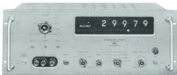
Fig. 3. Dymec 2401A Integrating Digital Voltmeter has floated and guarded input to achieve very high common-mode noise rejection. Most sensitive range of voltmeter is 0.1 volt full scale with resolution of 10 microvolts. Over-ranging of 300% is provided.
