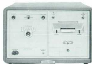
Fig. 2. New -hp- Model 562A Digital Recorder prints up to 3600 digits per minute on paper tape. Optional analog circuitry occupies left portion of panel.
