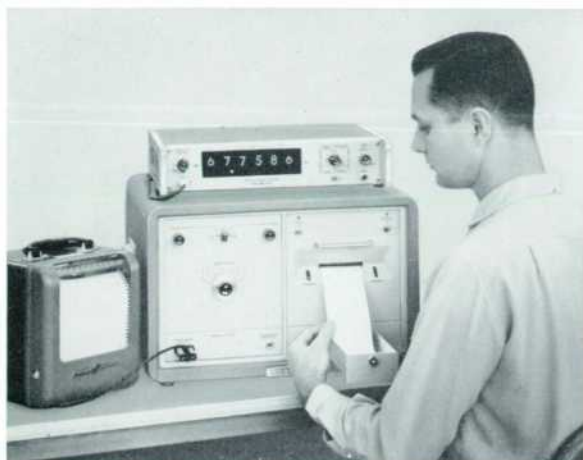
Fig. 1. New -hp- Model 562A Digital Recorder (center) operates from BCD codes to print digital data such as from counters on paper tape. Unit also has option of analog output to drive strip recorders.
