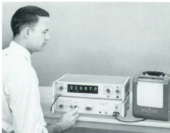
Fig. 1. New hp -Model 580A D-A Converter (lower center) enables digital data such as frequency counter readings to be recorded on either galvanometer or potentiometer type recorders.
