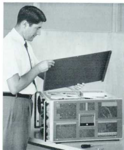
Fig. 9. All tubes can be replaced from top or bottom of instrument. Top and bottom covers can be removed in seconds.
