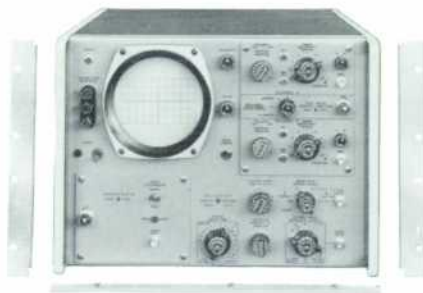
Fig. 10. Oscilloscope is provided with brackets that quickly convert the standard instrument into a rack-mountable unit.
