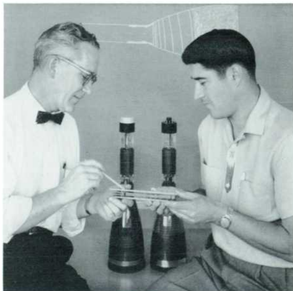
Fig. 11. Gun and deflection plate assembly used in new crt is discussed by William Kruger, tube designer and -hp- manager of crt development, and Floyd Siegel, project leader for Model 175A Oscilloscope.
