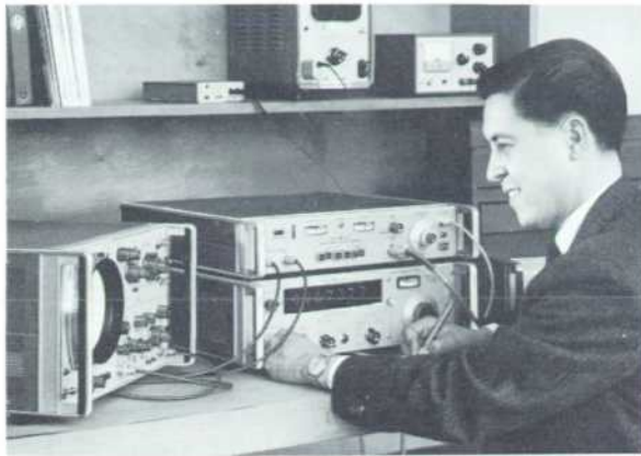
Fig. 6. Microwave Frequency Converter phase-locks built-in transfer oscillator to sub-multiple of microwave input frequency. Counter reads transfer oscillator frequency with characteristic precision. Converter permits measurement of frequencies of CW, FM, AM, and pulsed RF signals.
