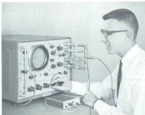
Fig. 1. New Model 188A dual-channel plug-in for -hp- Sampling Oscilloscope permits viewing signals of 90 picoseconds rise time, i.e., to above 4 gigacycles in frequency (to 8 Gc at reduced sensitivity). Plug-in is designed to view signals on 50-ohm lines by bridging line so that measured circuit is not disrupted.
