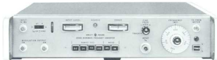
Fig. 5. Hewlett-Packard Model 2590A Microwave Frequency Converter enables accurate counter measurements of microwave frequencies in 0.5 to 15 Gc range. Built-in roll-chart (upper left) simplifies determination of frequency. Converter also has AM and FM demodulators to provide additional information about measured signals. Transfer oscillator may be used independently as 240-390 Mc signal source.
