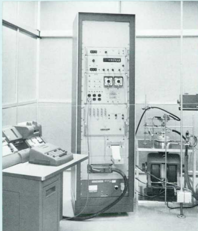
Fig. 1. The complete ADAC system consists of the controller and data-acquisition equipment in the rack and the dewar and magnet, shown at the right. This relatively compact system can be supplemented by various data-recording means, such as the card punch equipment, left.
