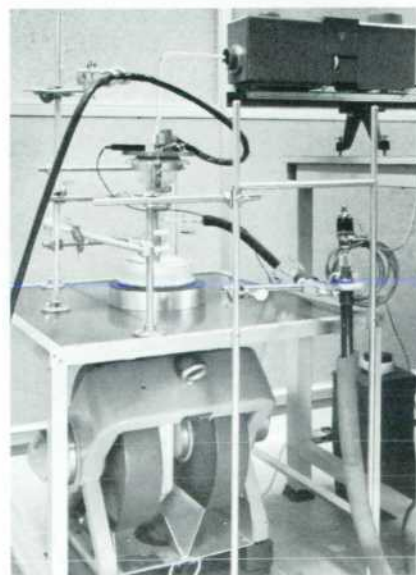
Fig. 3. Samples of materials are placed in a dewar. An electromagnet supplies the necessary magnetic field. Light is piped into the sample holder for photoconductivity and photo-Hall effect measurements.
