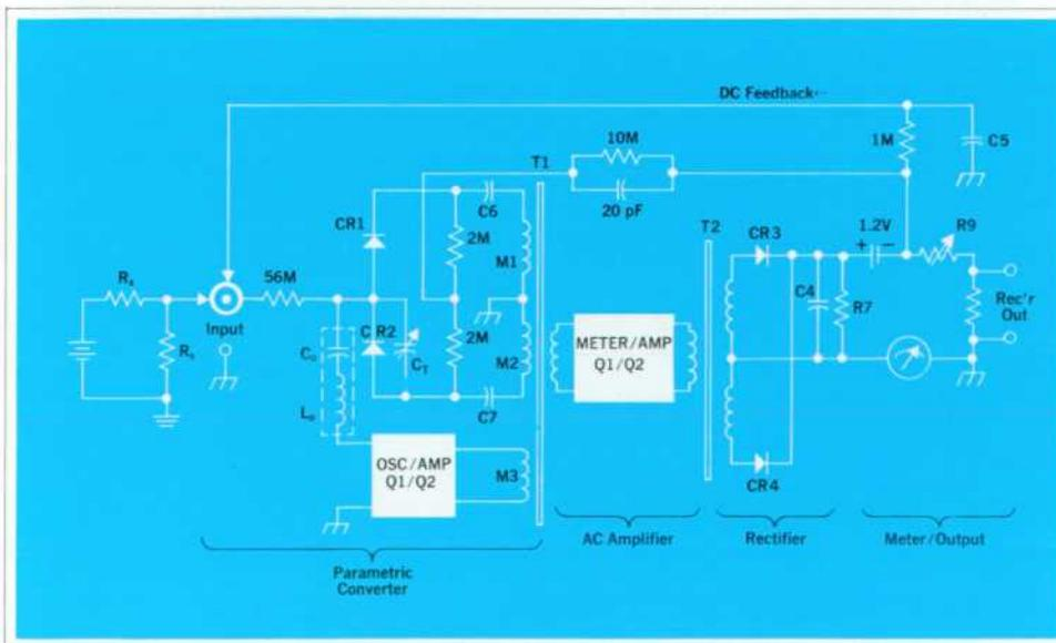
Fig. 8. A simplified circuit of the Model 4329A High Resistance Meter. Capacitor C<sub>T</sub> is the electrical zero adjust. It adjusts the oscillator output level to cancel the ±1.2 volt dc bias.
