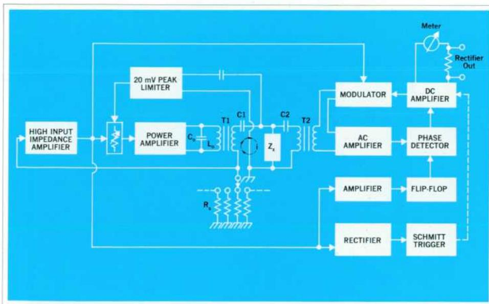
**Fig. 2.** Functional block diagram of the Model 4328A shows how a feedback loop is formed when  $Z_x$  is plugged in. Inductance of the primary winding of T1 and  $C_o$  determine the frequency of oscillation. The modulator prevents the meter voltage ( $V_x$ ) from varying in the presence of small changes in feedback loop or oscillator output.
