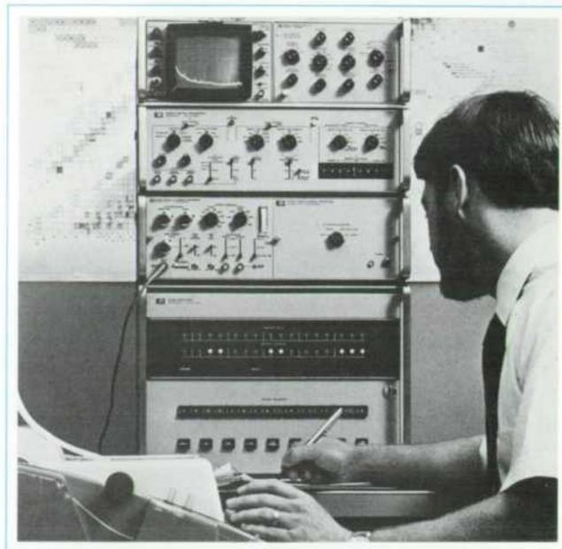
**Fig. 5.** HP 5402A MCA/BASIC System consists of analyzer, general-purpose digital computer, teleprinter, and interfaces. BASIC-language programming makes the system easy to operate. The analyzer and computer can be used separately or together as a system with the computer controlling the analyzer and doing data reduction.
