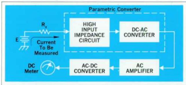
Fig. 5. Basic principle of the measuring technique used for high resistance measurements.
