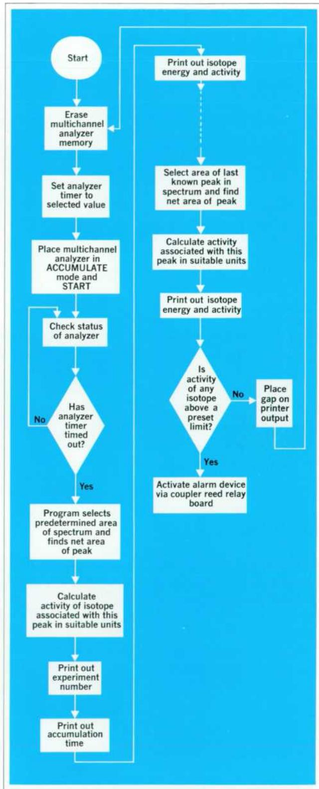
**Fig. 4.** Flow chart of calculator program for analysis of gamma-ray spectrum by HP 5403A MCA/Calculator System. The calculator controls the analyzer, computes the activity of all known isotopes in the sample, and triggers an alarm if the activity of any isotope is above a limit.
