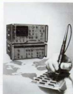
**Cover:** *The two subjects on this month's cover are symbolic of the broad range of Hewlett-Packard's electronic test capabilities. The Logic Pulser on the right simplifies checkout of microcircuit logic, right down to the individual gate. The Microwave Link Analyzer on the left checks out the performance of communications macrocircuits, all the way up to systems that span the world via satellite.*
