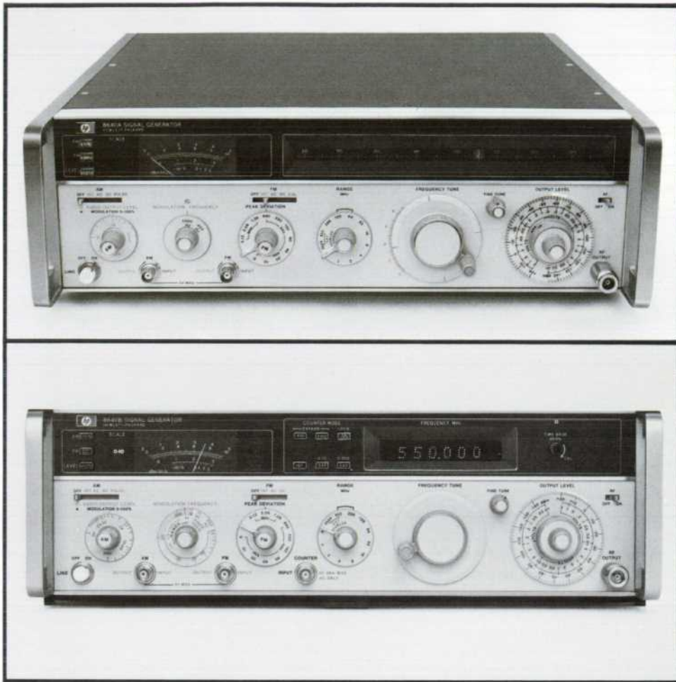
Fig. 2. Model 8640B Signal Generator is identical to Model 8640A in range of capabilities but also includes 550-MHz Counter for highly accurate frequency setting. In addition, Model 8640B has phase-locking to give crystal stability to output signal. Unit shown here also has optional audio oscillator.
