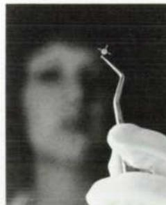
**Cover:** *The tweezers hold a new monolithic silicon-on-glass diode quad — four Schottky-barrier diodes arranged in a ring configuration (shown prior to encapsulation) for double-balanced mixer service. This construction achieves better matching and lower parasitics than has been possible with discrete components. For a description of this and another interesting diode development, see the article beginning on this page.*
