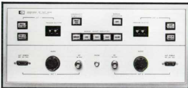
Fig. 4. Transceivers to be tested are connected to this RF test head. Two units at a time can be connected; one can be warming up while the other is being tested. A 15-foot cable allows the test head to be inside a screen room while the system remains outside.
