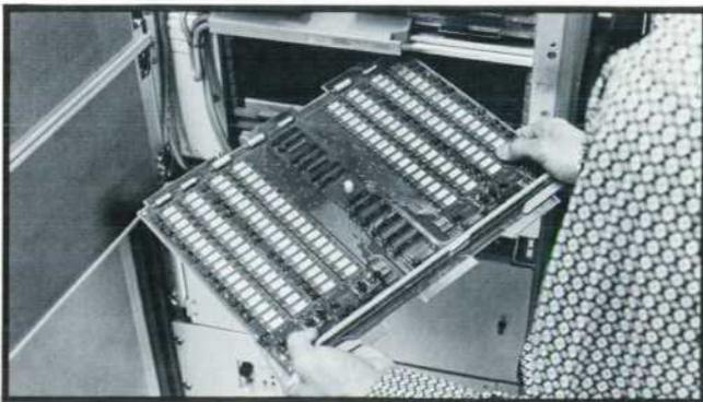
**Fig. 1.** 136 18-pin 4K RAMs on each HP 3000 Series II memory board provide 32,768 17-bit words of semiconductor memory capacity, four times the capacity of the same-size board with core memory. Series II memory is 50% faster and less than one-third as costly as the older core memory.
