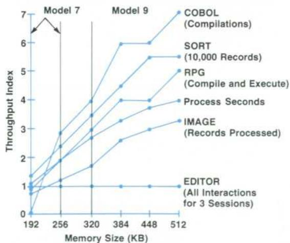
Fig. 1. Relative throughput of HP 3000 Series II models 7 and 9 using several measures of throughput. The base is a model 5 system with 128K-byte memory.
