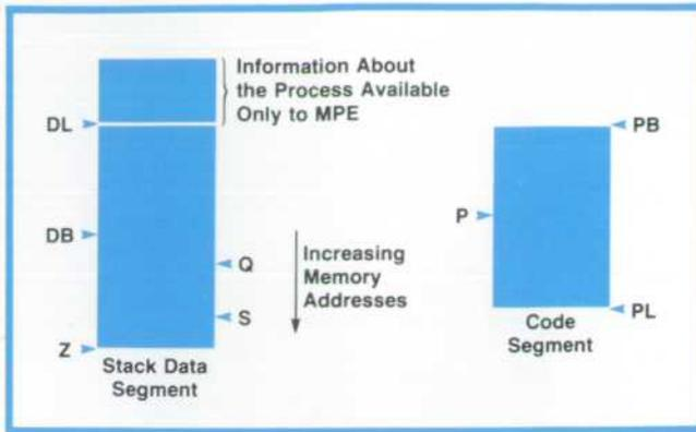
Fig. 2. Basic HP 3000 register structure. Memory is divided into variable-size segments of code and data. DL, DB, Z, Q, S, PB, PL, and P are registers that delineate various areas of the code and data segments.
