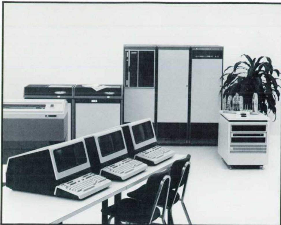
**Fig. 1.** Model 9, the largest HP 3000 Series II system, has the capabilities of a small-to-medium full-scale general-purpose computer, but is much lower in cost. It can meet the needs of larger commercial or scientific users. Model 7, a smaller system, is especially appropriate for users of small business computers who want to move upwards to on-line data base management. Model 5, the smallest Series II system, is a low-cost terminal-oriented system that also does concurrent batch processing.
