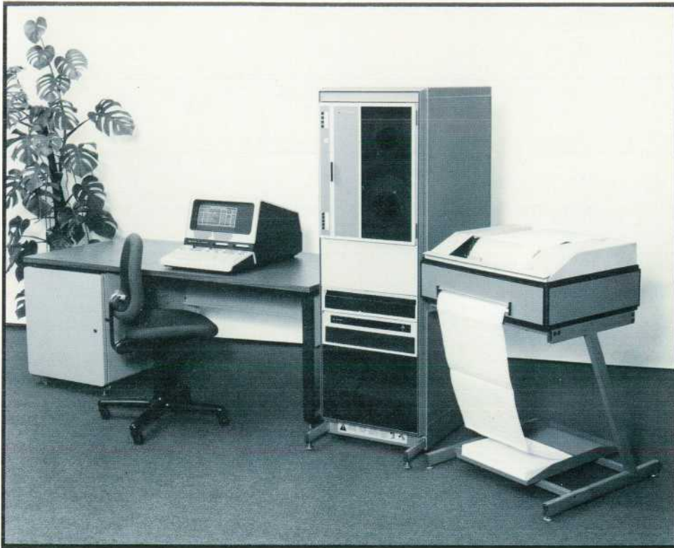
Fig. 2. HP 1000 Model 80 is a larger system suitable for data base management, operations management, and service as a central computer in a distributed system. Model 81 is the same system in two upright cabinets.
