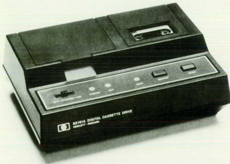
Fig. 1. The HP 82161A Digital Cassette Drive is a compact battery-operated mass-storage unit designed for use in portable HP-IL systems.
