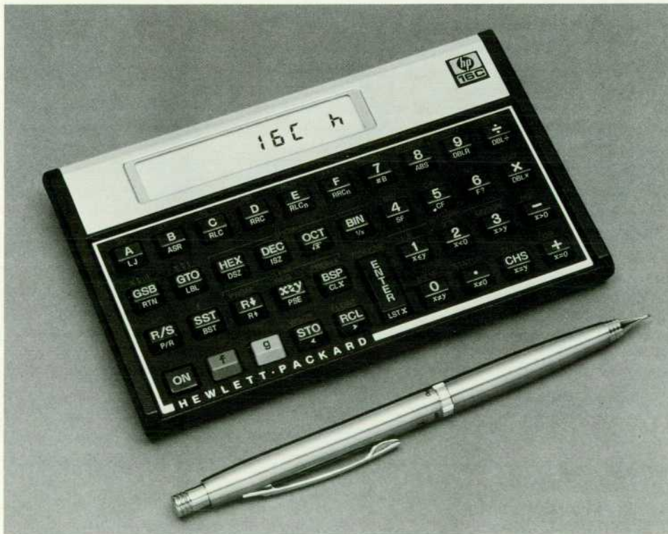
Fig. 1. The HP-16C Programmable Calculator is designed for computer science and digital electronics applications. Besides the normal four-function calculator features, it has a number of capabilities for setting number bases and word sizes, performing Boolean operations, and manipulating bits.
