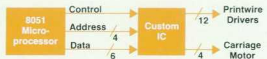
Fig. 1. The custom IC used in the HP 293X Printers interfaces the controlling microprocessor in these printers with their printhead and its carriage drive motor.
