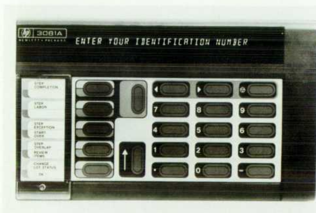
Fig. 1. The HP 3081A Industrial Workstation Terminal is sealed against dust and liquids to an IP rating of 65. The standard numeric keypad has large keys that are easy to operate with gloves on.
