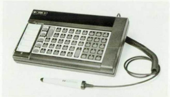
Fig. 2. Options include an alphanumeric keypad, a choice of bar code wands, and a choice of slot readers.
