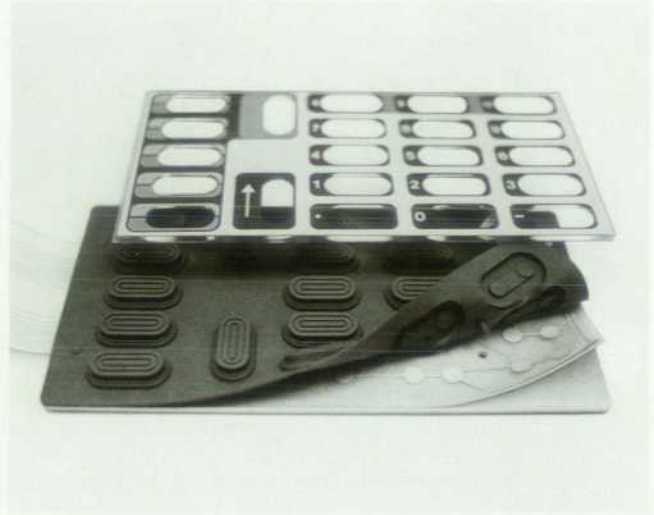
Fig. 10. The keyboard assembly consists of an elastomer keyboard that also functions as a gasket to seal the top case, a switch membrane circuit, a holder plate, and an overlay.
