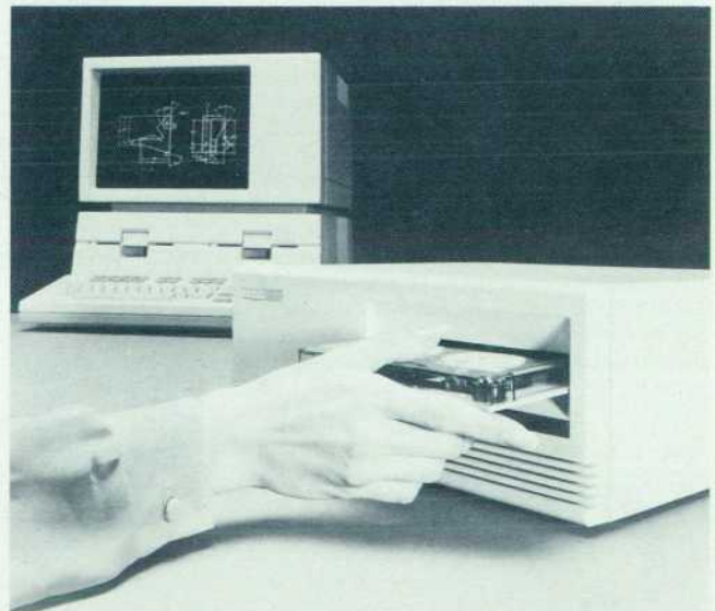
Fig. 1. The HP 9144A 1/4-Inch Cartridge Tape Drive offers convenient, low-cost backup of 67 megabytes on a single cartridge. Read after write capability and exclusive-OR error correction provide improved data reliability.
