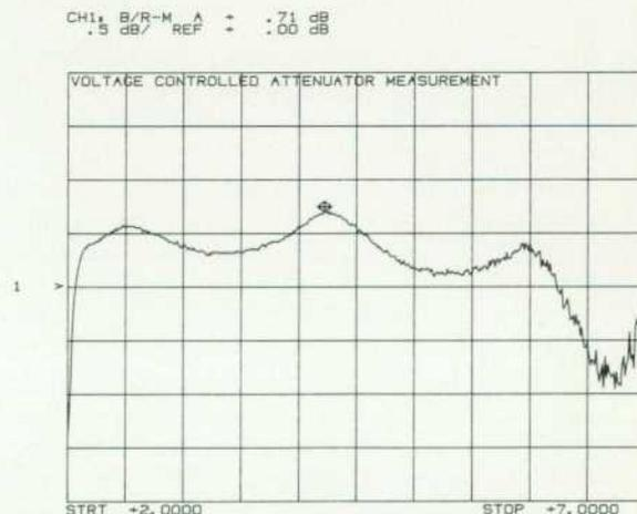
**Fig. 3.** Voltage-controlled attenuator linearity measurement. This is the same measurement as in Fig. 2, except that here the linear slope characteristic was removed by placing a sloped limit line into memory and selecting the measurement minus memory function.
