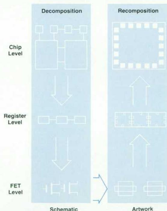
Fig. 1. Hierarchical block design (HBD) design flow.
