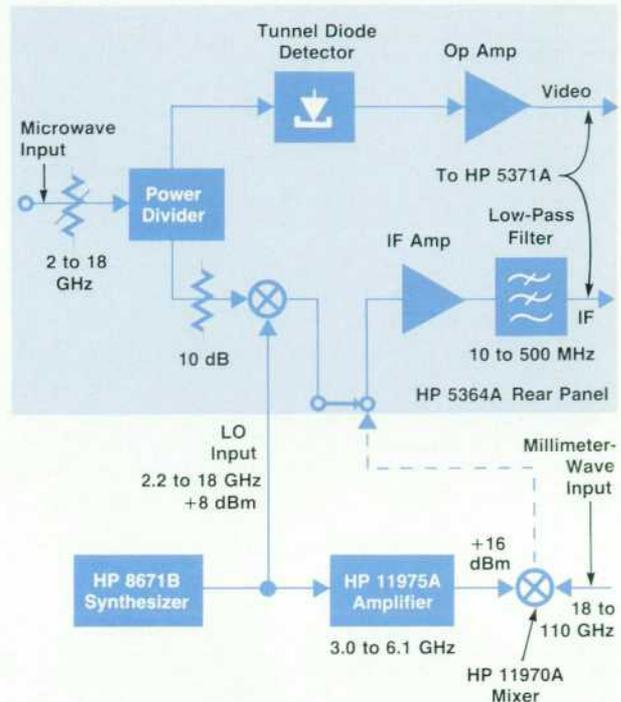
**Fig. 1.** The HP 5364A Microwave Mixer/Detector is used with an external local oscillator to down-convert microwave signals for analysis by the HP 5371A Frequency and Time Interval Analyzer. For millimeter-wave signals, an external mixer is also required.
