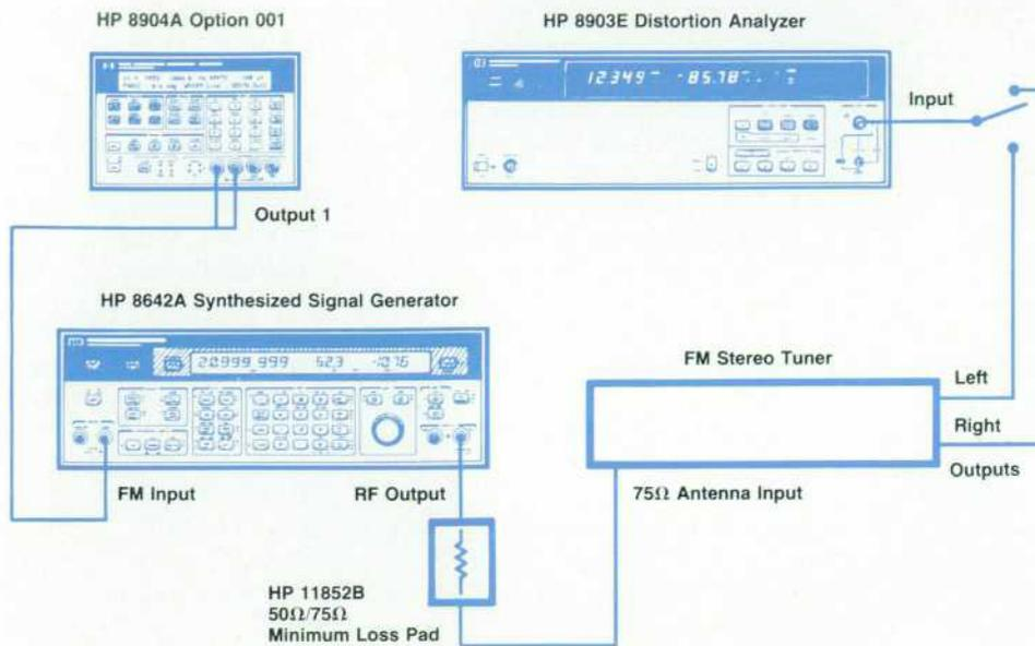
Fig. 2. Test setup for performance testing of an FM stereo receiver using the HP 8904A.
