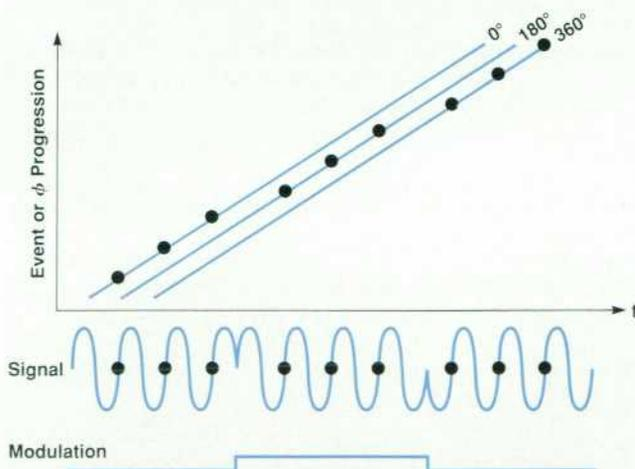
Fig. 8. Phase progression plot for a BPSK signal.
