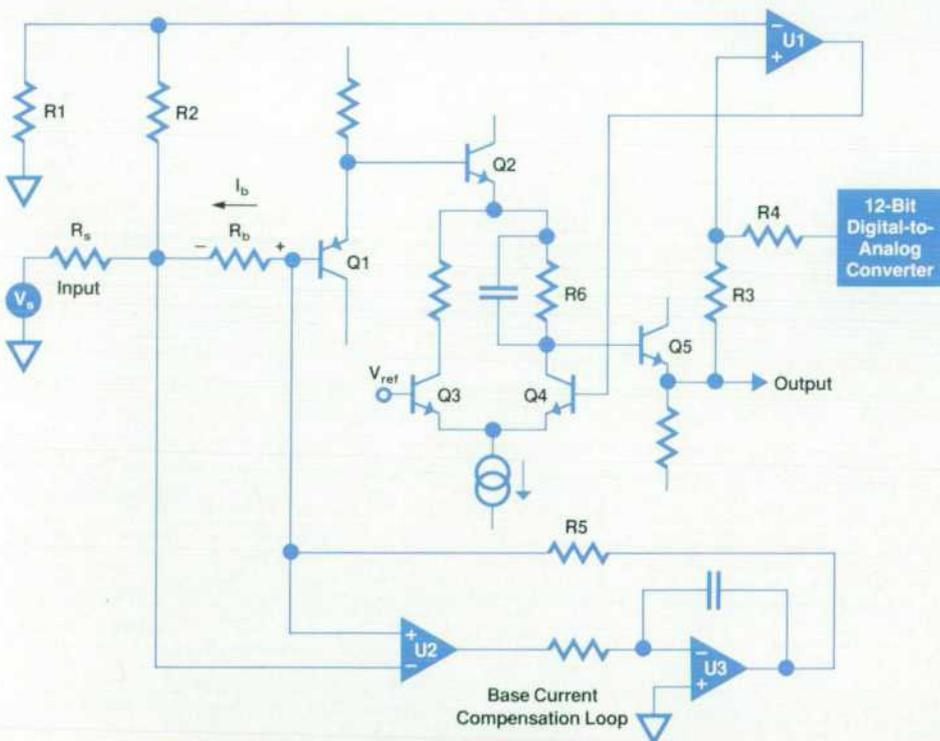
Fig. 2. Simplified diagram of the dc offset circuit.
