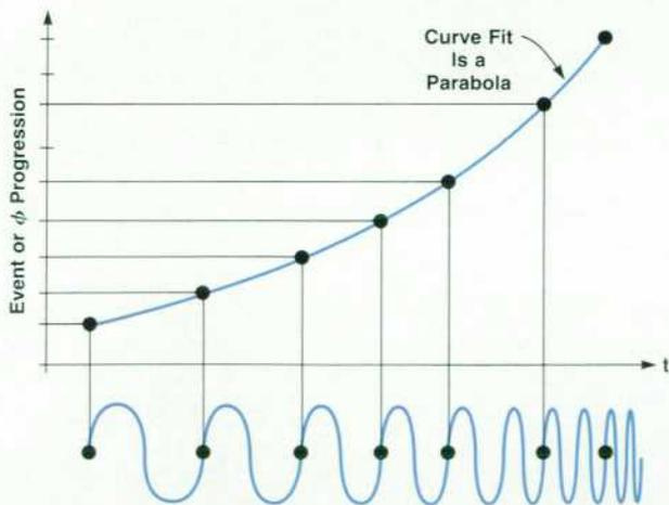
Fig. 6. Phase progression plot for a linear frequency chirp.
