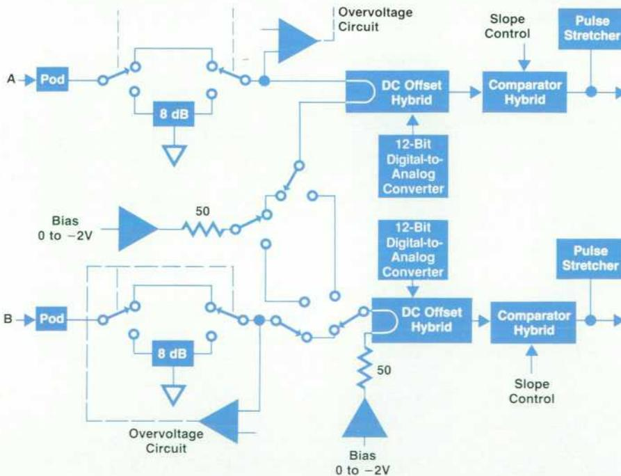
**Fig. 1.** Simplified block diagram of the input amplifier of the HP 5371A Frequency and Time Interval Analyzer.
