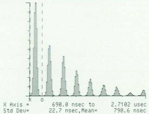
Fig. 10. Histogram of compact-disc pulse width measurements with eight-of-fourteen modulation.
