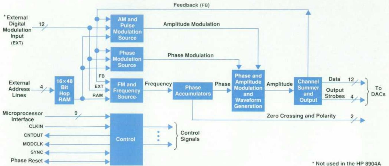
Fig. 1. Digital waveform synthesis IC block diagram.
