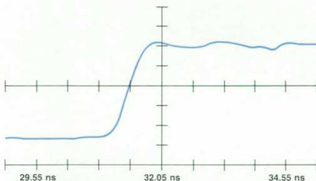
Trigger is free-running at 500 kHz with step on.
