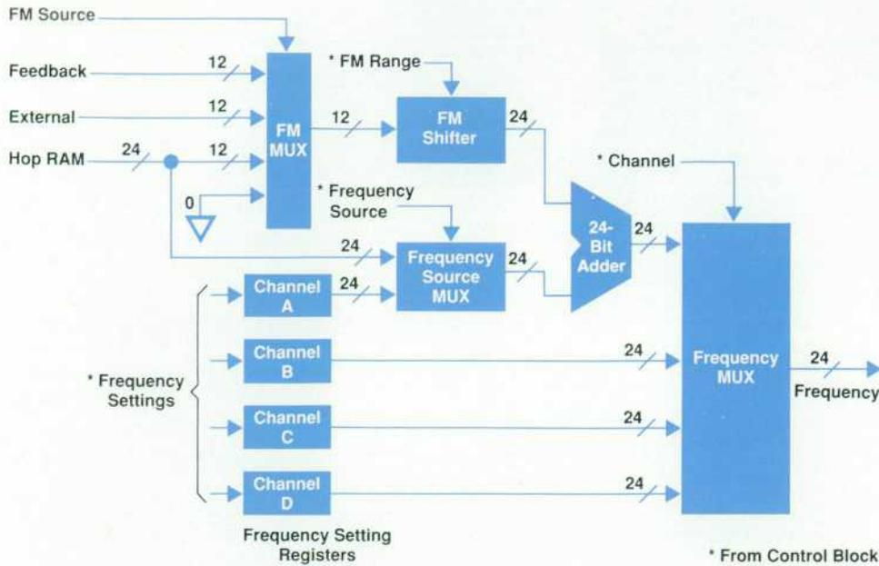
\* From Control Block **Fig. 5.** FM and frequency source.
