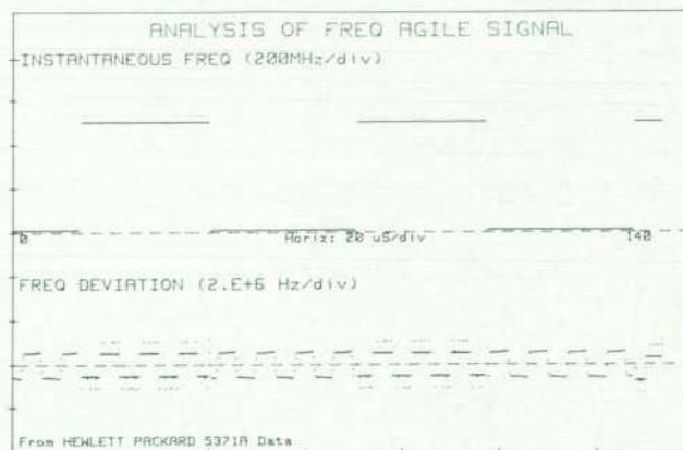
Fig. 4. A measurement of FSK modulation on a frequency-hopped carrier.
