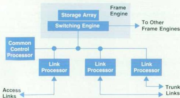
Fig. 6. Network node structure.
