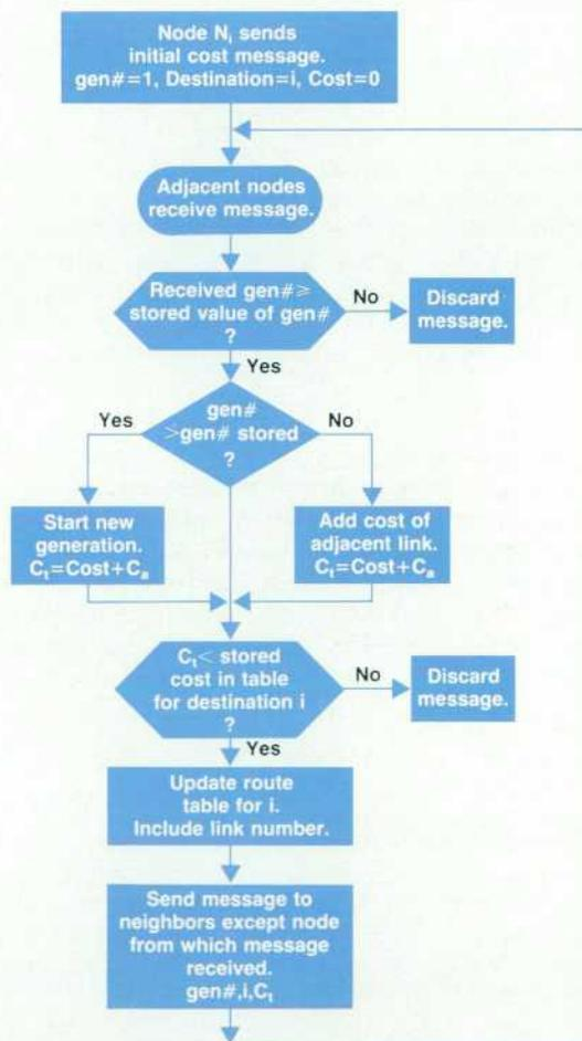
Fig. 12. Routing algorithm.
