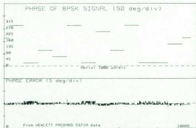
Fig. 9. Phase and phase error of an 8PSK signal.
