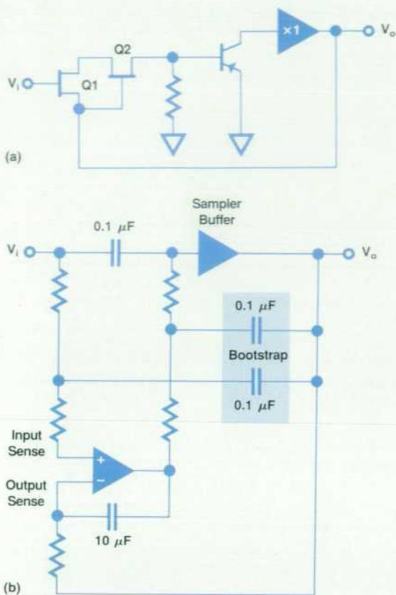
Fig. 3. (a) Sampler buffer. (b) Dc correction loop.
