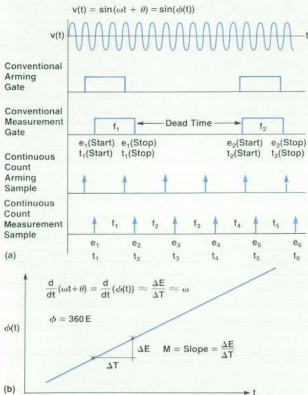
**Fig. 2.** (a) A comparison of reciprocal counter operation and the continuous count technique. In continuous counting, the stop sample of one measurement is the start sample of the next. Measurements are made in blocks, and there is no dead time within a block. (b) The reciprocal counter estimates frequency as the derivative of phase, that is, the slope of a straight line connecting the start and stop sample values.
