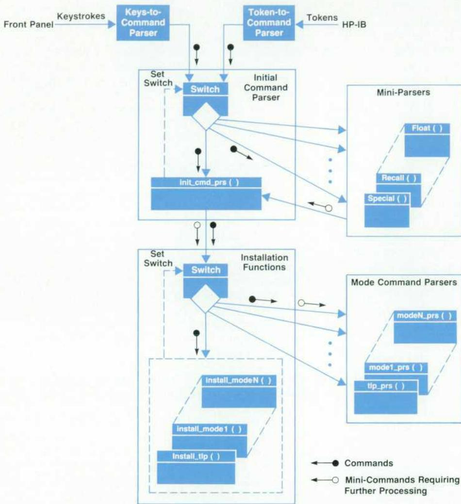
Fig. 2. Command parsing structure for the HP 8904A.
