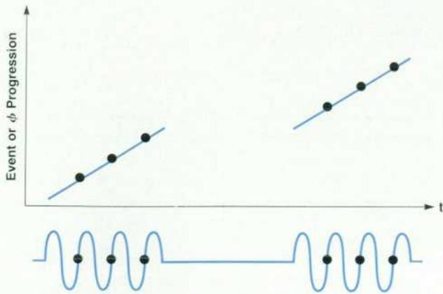
Fig. 5. Phase progression plot for pulsed RF.
