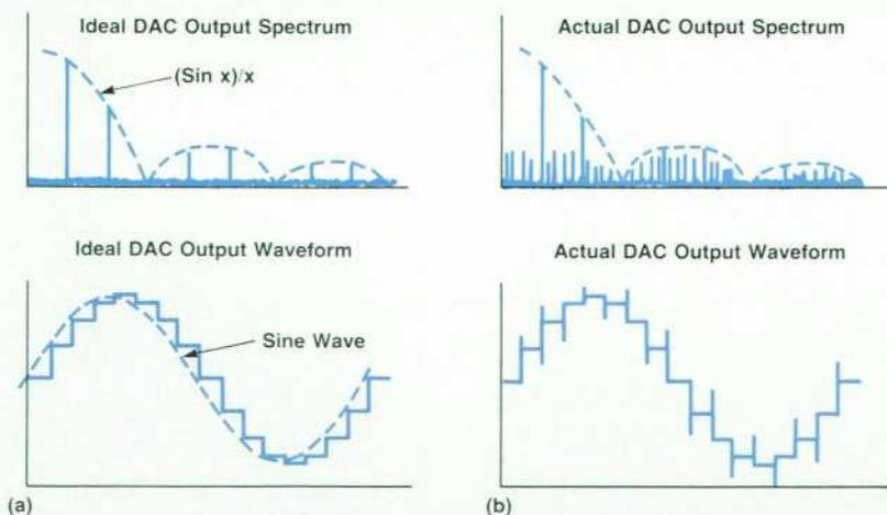
**Fig. 1.** (a) Ideal DAC output spectrum and ideal DAC output waveform. (b) Actual DAC output spectrum and actual DAC output waveform.
