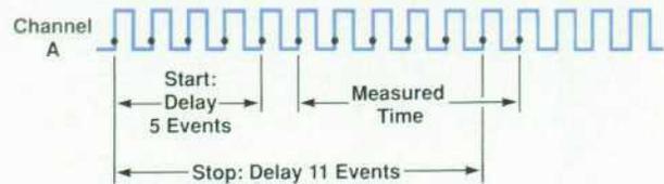
Fig. 7. The start and end of a single measurement can both be defined by time or event holdoffs.
