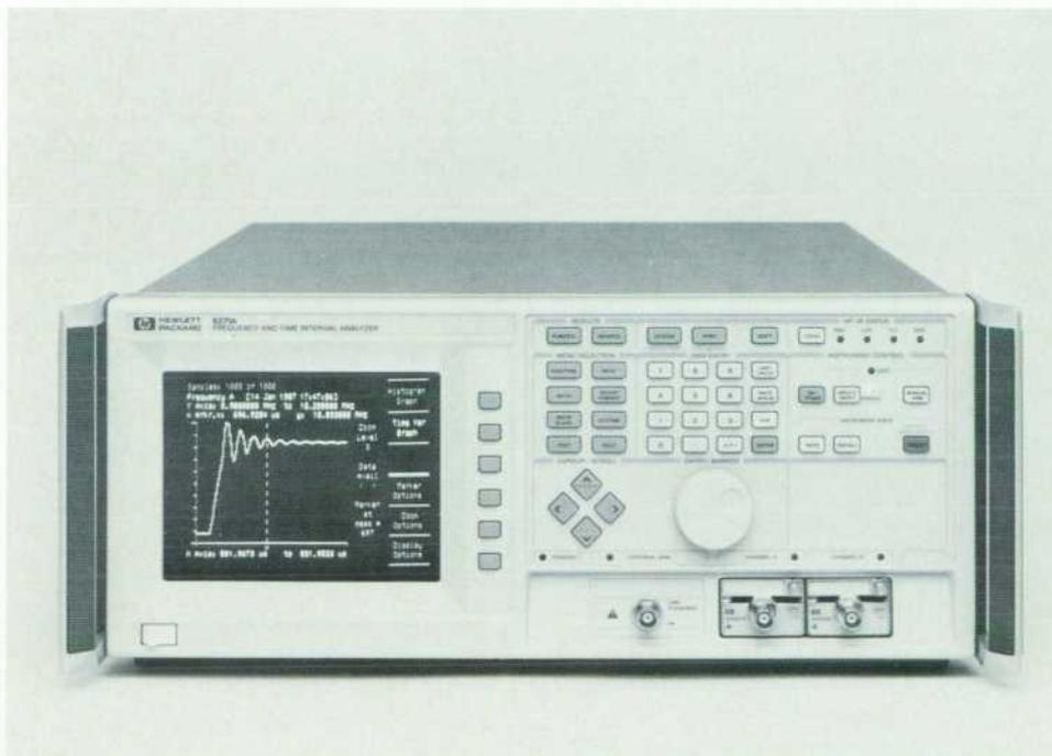
**Fig. 1.** The HP 5371A Frequency and Time Interval Analyzer provides new capabilities for characterizing the frequency behavior of agile and other time varying sources. Its frequency range is dc to 500 MHz, but its capabilities can be applied to signals in the 2-to-18-GHz range using the HP 5364A Microwave Mixer/Detector.
