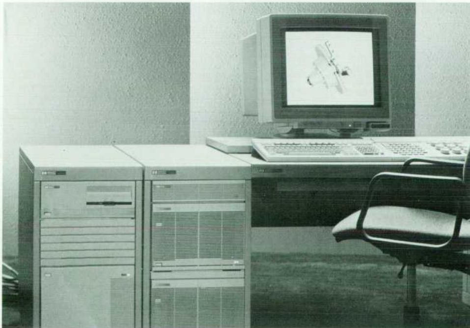
Fig. 2. The HP 9000 Model 835 TurboSRX is a 3D solid-rendering graphics superworkstation with animation capability. Like other Model 835 multiuser technical computers, it runs the HP-UX operating system.
