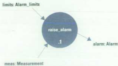
Fig. 2. Initial data flow diagram of the raise_alarm process.
