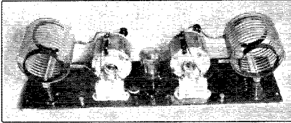
A VIEW OF THE LOW-POWERED TUNED GRID-TUNED PLATE TRANSMITTER WHICH MAY BE USED AS IS OR AS A MASTER OSCILLATOR FOR A 50-WATT AMPLIFIER
