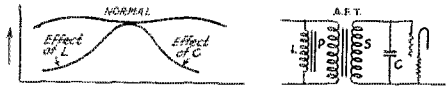
FIG. 9. THE EFFECT OF A PRIMARY SHUNT CHOKE AND A SECONDARY SHUNT CAPACITY IN PRODUCING PEAKS AND HIGH OR LOW CUTOFFS.
