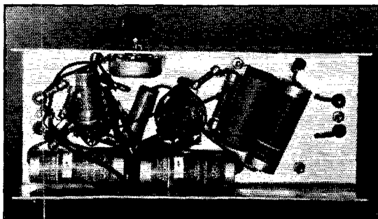
RESISTORS AND CONDENSERS ARE PUT IN THE MOST CONVENIENT LOCATIONS UNDERNEATH THE MODULATOR CHASSIS
