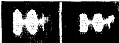
(Left) OSCILLOGRAPH OF A CLASS-B LINEAR AMPLIFIER WHEN THE EXCITATION IS TOO HIGH
