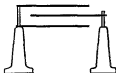
Fig. 3—The tuning condenser is simple to make and inexpensive as shown by this sketch.
