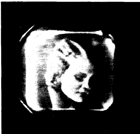
Actual-size unretouched photograph of the 120-line image appearing on the 902 monitor screen.
