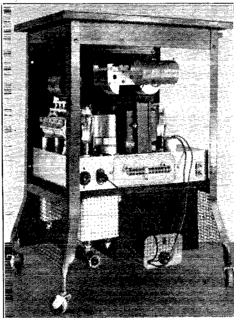
Wire screening of the power supply and bleeder resistor is well shown in this rear view of the transmitter installation, as well as the power connections between the units. The inverted 866 rectifiers are between the lower front panel and the power transformer.
