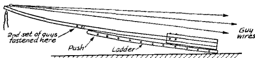
Fig. 3 — W2JAW uses a ladder to brace a light mast while it is being erected.
