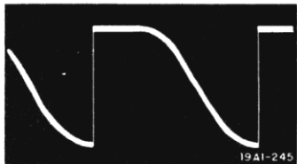
FIG. 51 TP13 VERT. PULSE Plate of Vertical Output Pin 2 of V15 (6SL7GT) 286 Volts PP
