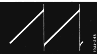
FIG. 49 TP11 VERT. PULSE Output of Vertical Oscillator Pin 5 of V11 (6SN7GT) 22 Volts PP
