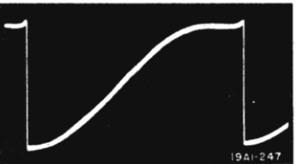
FIG. 53 TP15 VERT. PULSE Plate of Vertical Output Pin 5 of V15 (6SL7GT) 286 Volts PP
