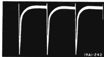
FIG. 48 TP10 VERT. PULSE Input to Vertical Oscillator Pin 4 of V11 (6SN7GT) 76 Volts PP
