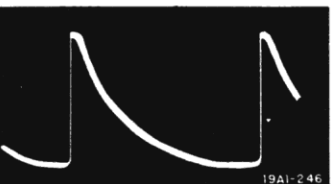
FIG. 52 TP14 VERT. PULSE Grid of Vertical Output Pin 4 of V15 (6SL7GT) 7 Volts PP
