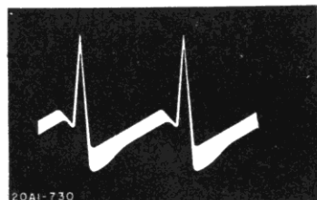
Fig. 64A 9 Volts PP Plate of Hor. Sync *TP13A Disc V404 (6AL5) Pin 2 in sets with 12AU7 (V403) Pin 7 in sets with 6AU6 (V403)
