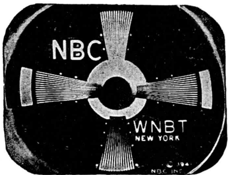
Figure 3-4—Test Pattern Excessive Contrast
