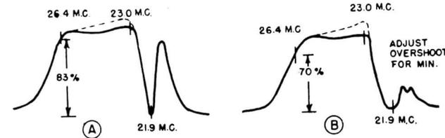
Fig. 9. Video I-F Alignment Curves
