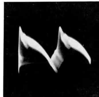
Figure 69. Cathode Waveform (Horizontal) at Pin 3 or 6 of Horizontal-Damping Tube
