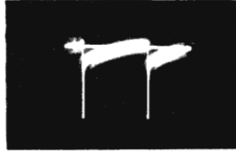
Figure 36—Grid of Vertical Oscillator Tube (175 Volts, P to P) (Pin 1 of V107)
