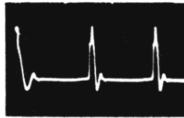
Figure 45—Plate of Horizontal Output (Approx. 5000 Volts, P to P) (Measured Through a Capacity Divider Connected from Plate to Ground)
