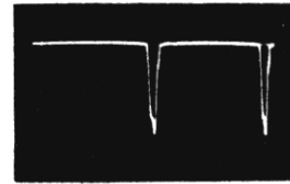
Figure 46—Voltage Across Horizontal Deflection Coils (Approx. 1100 Volts, P to P) (Pin 4 or 6 of V111 to Ground)
