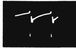
Figure 42—Grid of Horizontal Oscillator (400 Volts, P to P) (Pin 4 of V108)
