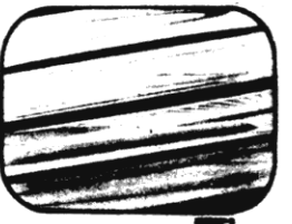
Figure 47—Test Pattern Showing Out of Sync Condition When Horizontal Hold Control Is in a Counterclockwise Position—Just Before Pulling Into Sync
