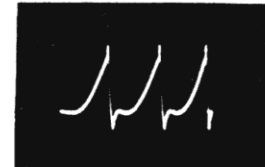
Figure 40—Horizontal Oscillator Waveforms and Sync Pulse (20 Volts, P to P) (Junction of C122 and C133)
