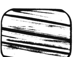
Figure 45—Plate of Horizontal Output (Approx. 5000 Volts, P to P) (Measured Through a Capacity Divider Connected from Plate to Ground)
