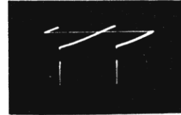
Figure 37—Input to Vertical Output Tube (65 Volts, P to P) (Junction of C129 and C130)
