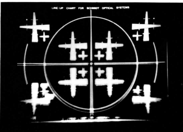
FIG. 7 - Lateral adjustment of optical barrel incorrect, as shown by a lack of a parallel condition of the vertical lines.
