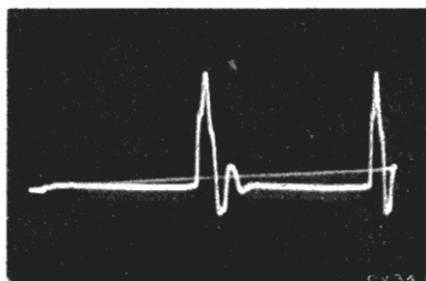
Figure 77—Plate of Horizontal Output (Approx. 6000 Volts PP) (Measured Through a Capacity Voltage Divider Connected from Top Cap of V126 to Ground)
