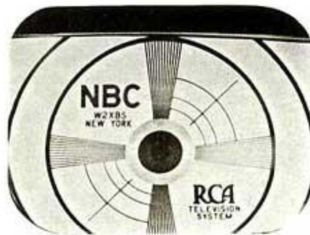
Figure 9—INCORRECT VERTICAL CENTERING To correct—Adjust Vertical Centering Control (screwdriver adjustment) to center picture vertically
