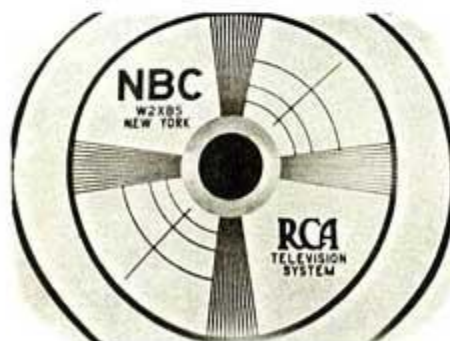
Figure 13—INCORRECT VERTICAL LINEARITY —(Circles flattened at top) To correct—Turn Vertical Linearity Control clockwise and Height Control counterclockwise (screwdriver adjustments)
