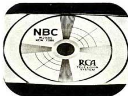
Figure 11—INCORRECT HEIGHT To correct—Adjust Height Control (screwdriver adjustment) for correct height of picture
