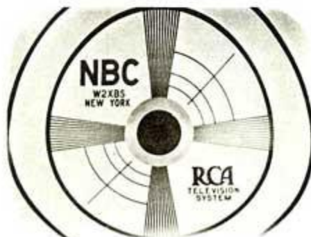
Figure 12—INCORRECT VERTICAL LINEARITY —(Circles flattened at bottom) To correct—Turn Vertical Linearity Control counterclockwise and Height Control clockwise (screwdriver adjustments)
