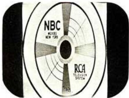
Figure 10—INCORRECT WIDTH To correct—Adjust Width Control (screwdriver adjustment) for correct width of picture
