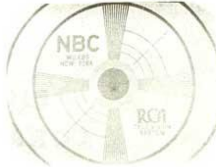
Figure 5—TOO LITTLE CONTRAST To correct—Turn Contrast Control clockwise and Brightness Control counterclockwise
