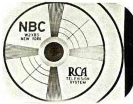
Figure 8—INCORRECT HORIZONTAL CENTERING To correct—Adjust Horizontal Centering Control (screwdriver adjustment) to center picture horizontally
